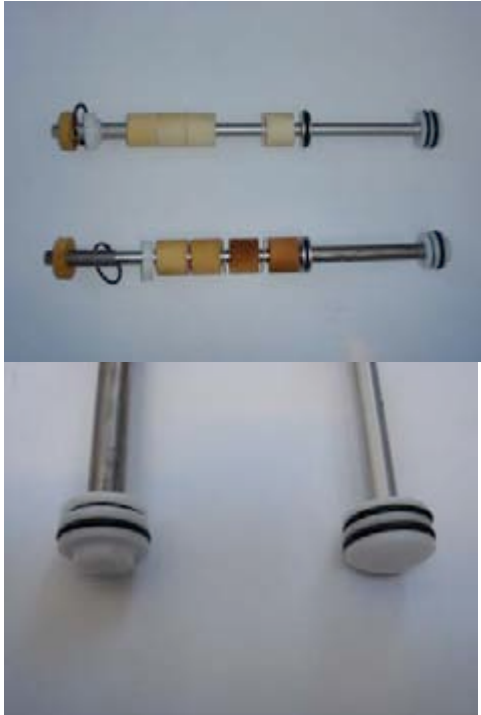
Top: Durin, bottom: XC air forks stepped piston
