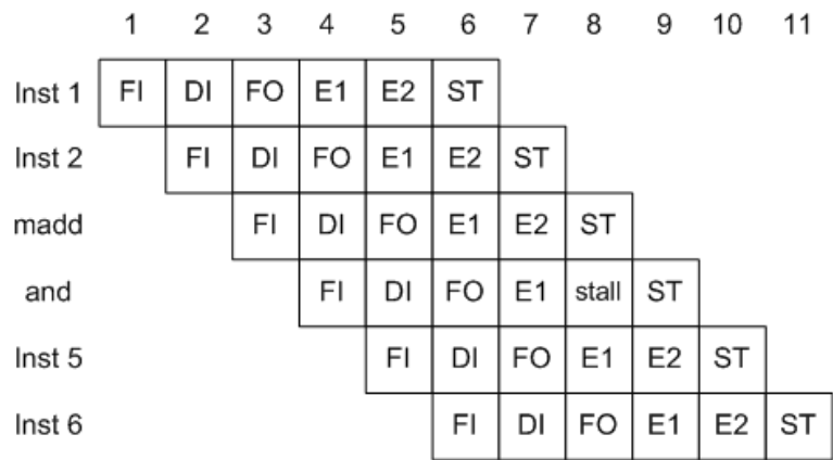
Figure 3.9: Pipeline data hazard
